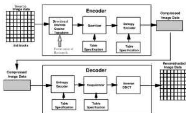
**Figure 1** - Block diagram of directional DCT based Image Compression system.
